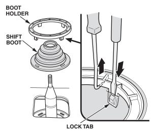
3. Pull up and remove the boot holder and the shift boot.
