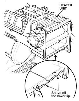
3. Remove the front screw from the bottom of the heater unit.
