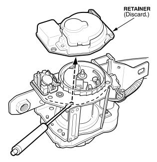
17. *Driver's side only:* If the retainer you removed is green, install the red cap from the kit on the retractor reel shaft. If the removed retainer is pink, do not install the cap.
