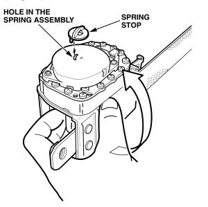
15. Turn the retractor assembly over, and use the small end of the pin punch from the kit to drive the three pins out of the retainer. Make sure the pins do not fall inside the retractor mechanism. Discard the pins.
