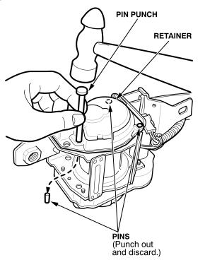
16. Use a small screwdriver to pry the retainer off the seat belt retractor assembly. Pry carefully along the edges. Do not stick the screwdriver too far under the retainer; you could damage the retractor mechanism. Discard the retainer.
