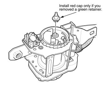
18. Remove the sensor from the retractor assembly with your fingers. Discard the sensor.
