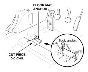
9. Install the driver's floor mat and place its grommet over the pin.
