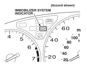
If you insert a nonprogrammed ignition key into the ignition switch and turn the switch to ON (II), the indicator comes on for **2 seconds** and *then starts to blink*. The indicator keeps blinking until you turn the switch to LOCK (0). If you try to start the engine with a nonprogrammed ignition key, the engine cranks, but it cannot start.
